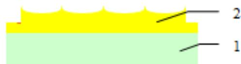
3. Anisotropic ion beam etched. The 3D micro-mirror array formed in the substrate.
