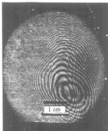
FIG. 2. Moiré fringes obtained by superposing patterns of Figs. 1b and c in a single exposure.
